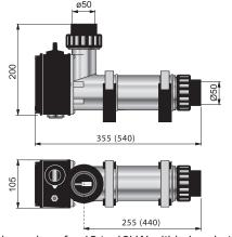
Dimensions for 12 to 18kW within brackets. Minimum flow 90 I/min
