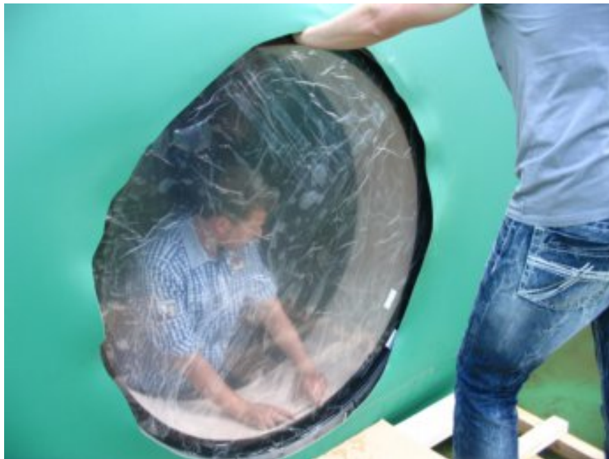
Abbildung 6: The window is lifted into the window opening
