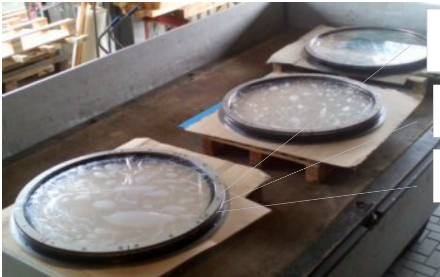
Abbildung 4: As an example the picture shows three round windows with pressure flange
