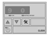
The first number on the LED screen stands for the number of the parameter and the second one for its value.
