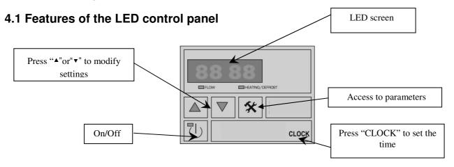
With the "On/Off" key "'\_」", the heat pump is turned on or turned off (stand-by status). If the LED next to this key lights up, the heat pump is turned ON.
